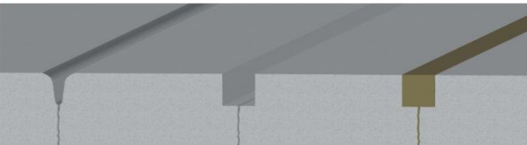
Repair random Cracks Fill and repair existing joint New construction joint protection
